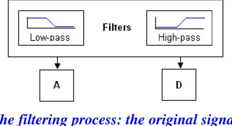
The filtering process: the original signal X passes through two complementary filters and emerges as two signals (A and D)
