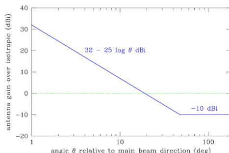
Figure 3. ITU-R SA.509 model of peak sidelobe levels for the VLBI and SLR radar antennas.
