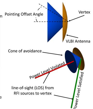
Figure 7. Geometric depiction of pointing angle offset requirement
