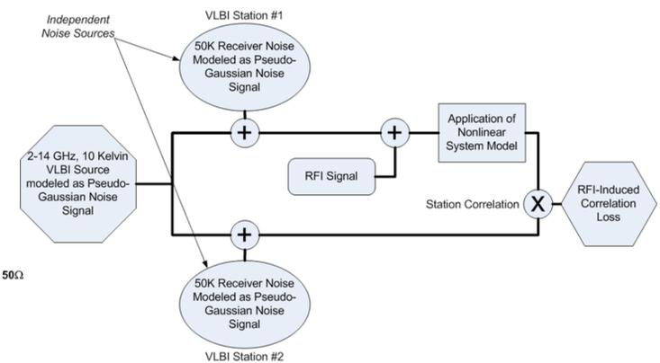
Figure 2. Block diagram outlining VLBI signal simulation used to assess station correlation loss
