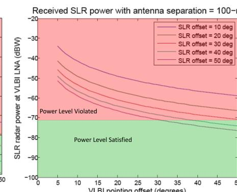
Figure 6. SLR radar Pointing Offset Requirements
