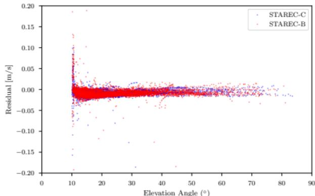
(b) Residuals w.r.t Elevation, per antenna type.
