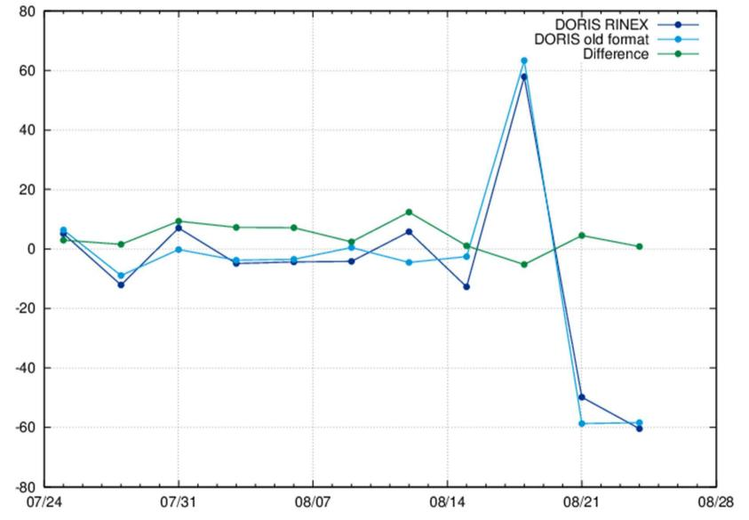
Figure on the left shows the dx helmert parameter in (mm) of the two SINEX solutions. Larger values for last three weeks caused by the SPJB station
