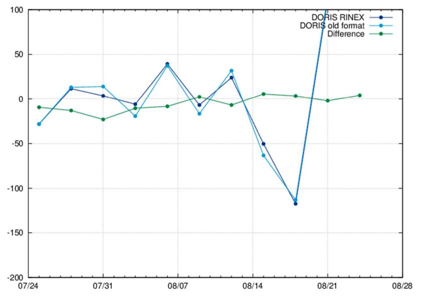
Figure on the left shows the dz helmert parameter in (mm) of the two SINEX solutions. Larger values for last three weeks caused by the SPJB station
