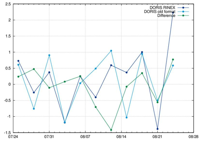
Figure on the left shows the scale helmert parameter in (ppb) of the two SINEX solutions. Larger values for last three weeks caused by the SPJB station
