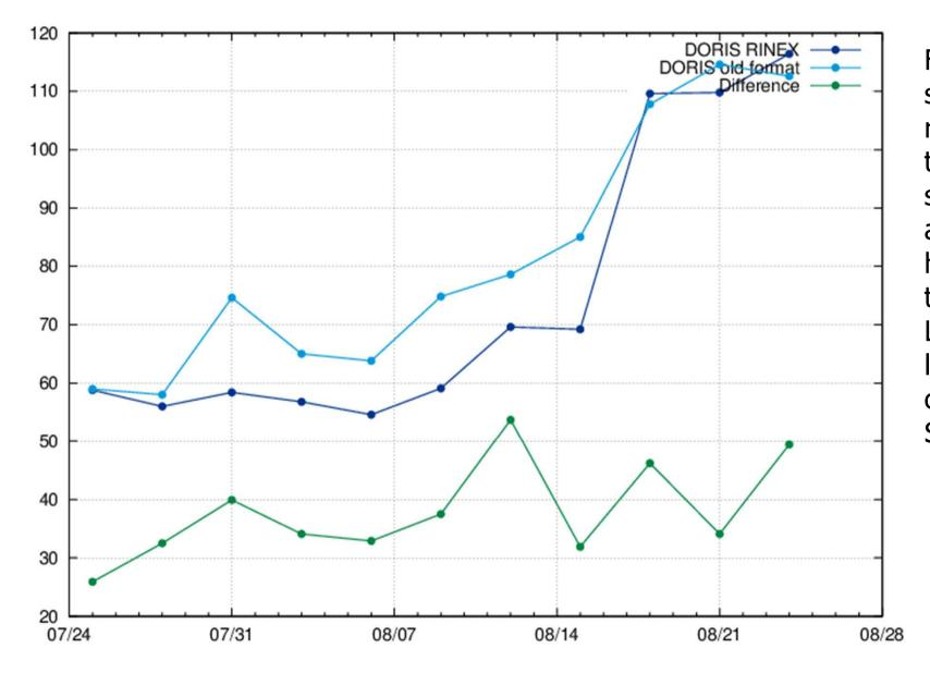
Figure on the left shows the weekly repeatability of the two SINEX solutions in (mm) after removing a helmert transformation. Larger values for last three weeks caused by the SPJB station
