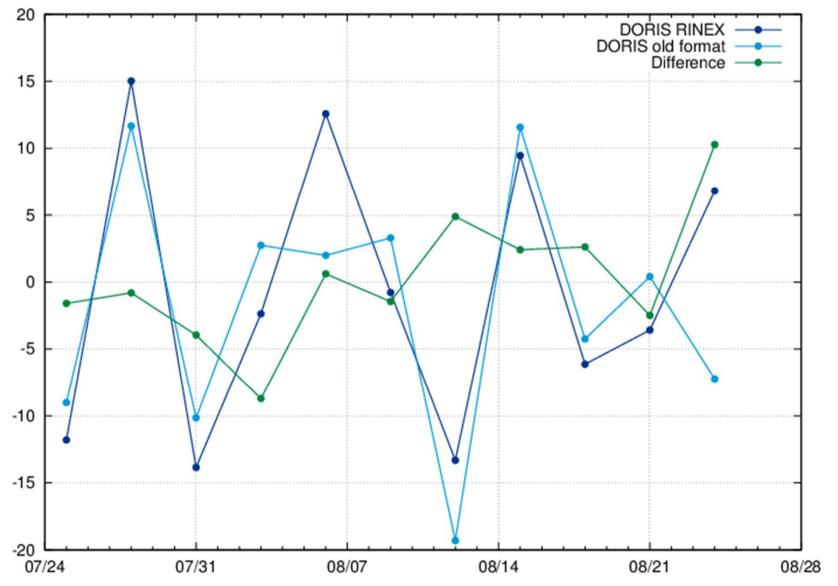
Figure on the left shows the dy helmert parameter in (mm) of the two SINEX solutions. Larger values for last three weeks caused by the SPJB station
