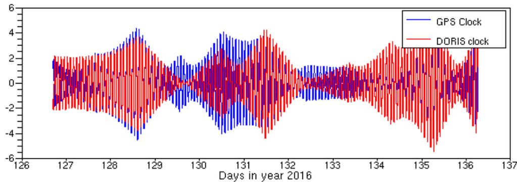
Radial orbit difference to GPS orbit (cm)
