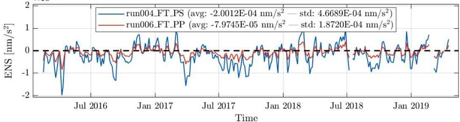
➔ Reduced scattering of POD parameters when estimating tropospheric refraction scale factors (SF) per pass.
