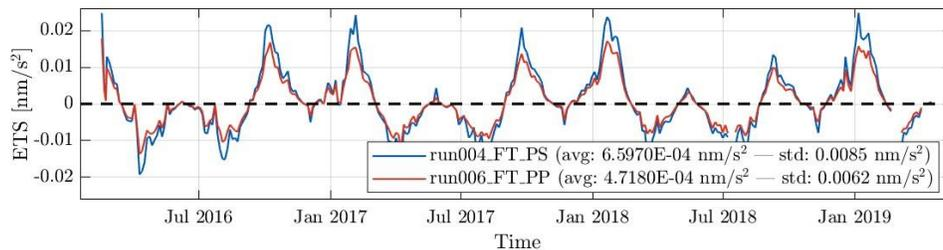
Jason-3: comparison of POD parameters of different solutions
