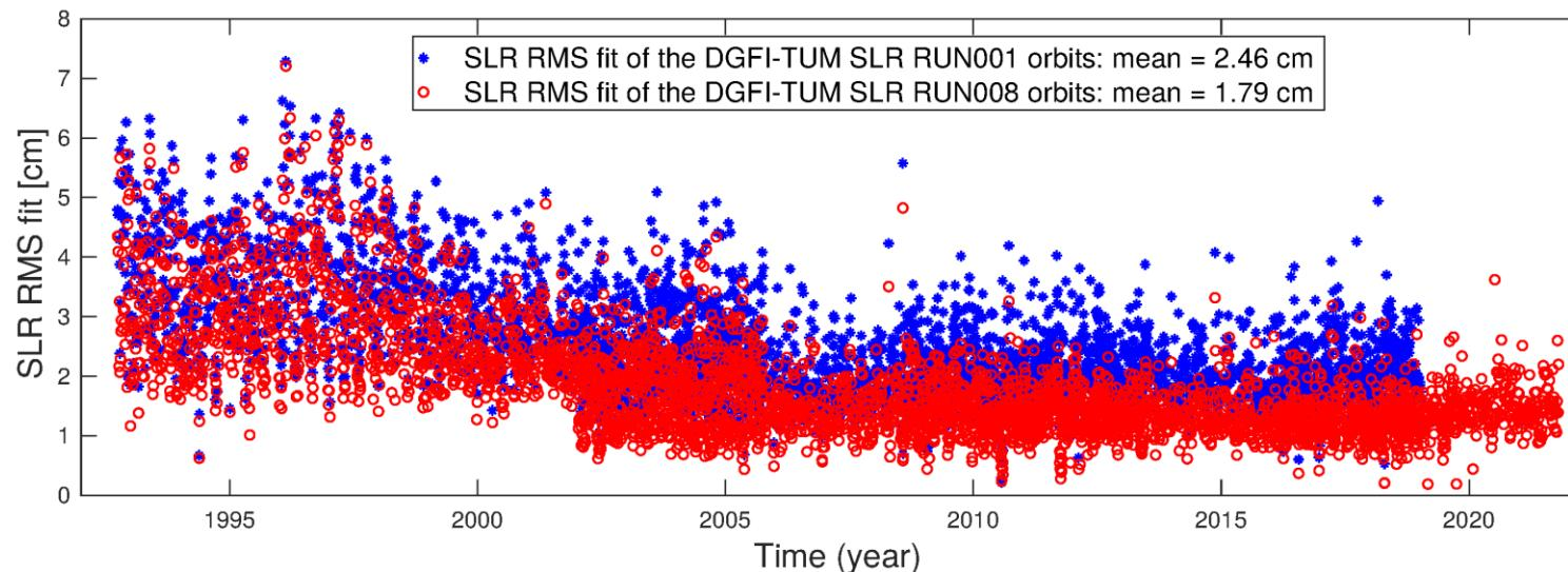
RMS differences of SLR observations of TOPEX/Poseidon, Jason-1, Jason-2, and Jason-3 of DGFI-TUM SLR RUN001 and RUN008 orbits.
