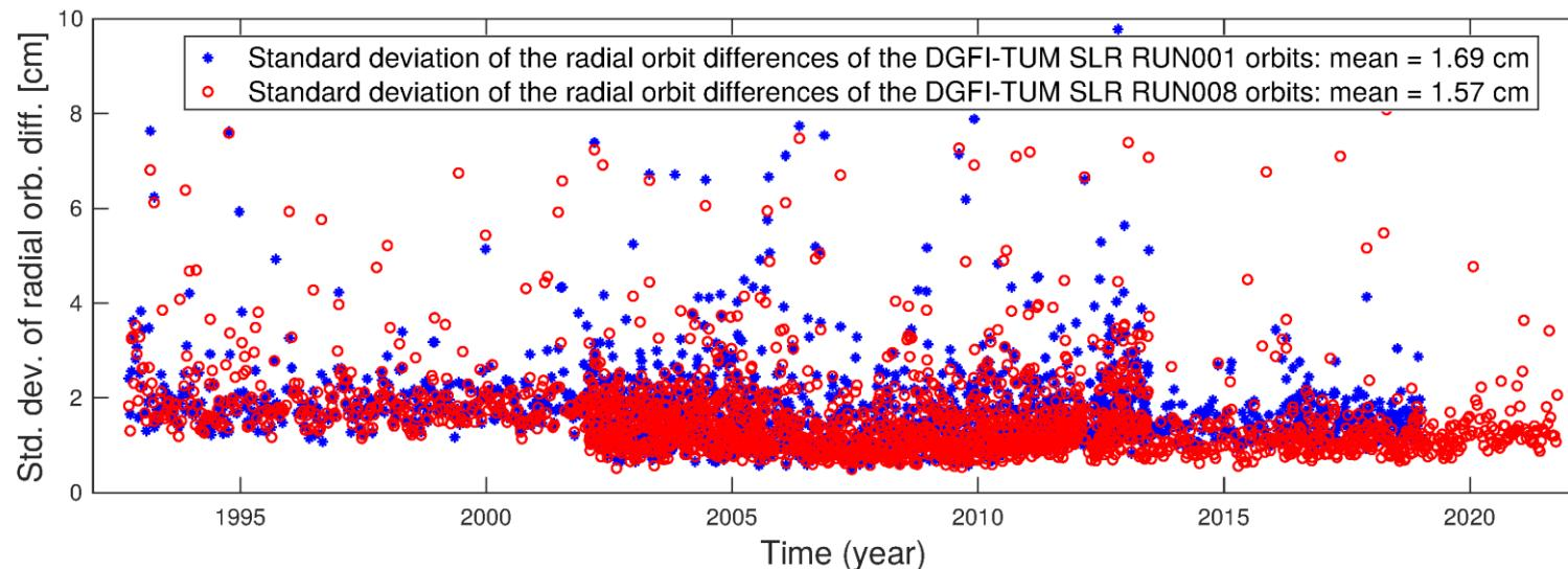
Standard deviation of the orbit differences in the radial direction of DGFI-TUM SLR RUN001 and RUN008 orbits with respect to GFZ VER13 orbits of TOPEX/Poseidon and Jason-1 and CNES POE-F orbits of Jason-2 and Jason-3.
