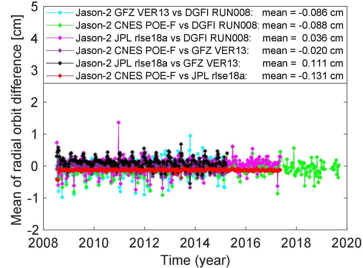
All orbits agree within 5-13 mm in RMS and  $\pm 1.3$  mm in mean. CNES POE-F, JPL and GFZ VER13 orbits agree within 5-8 mm in RMS. SLR data-only DGFI RUN008 orbit agrees within 12-13 mm in RMS with DORIS or GPS data derived orbits from CNES, GFZ and JPL.
