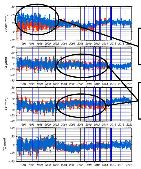
Scale difference until 2002.5 is due to the new ALCATEL antennae PCV.
