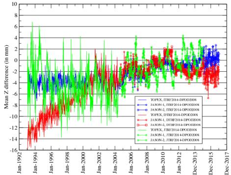
Orbit centering difference in the Z direction: • important drift from 1993 to 2001 for DTRF2014 • drift consistent between the 3 TRFs after 2002 • annual signal for JTRF2014 (weekly solution) • different geocenter than those of DPOD2008 • correlated to the Tz parameter differences
