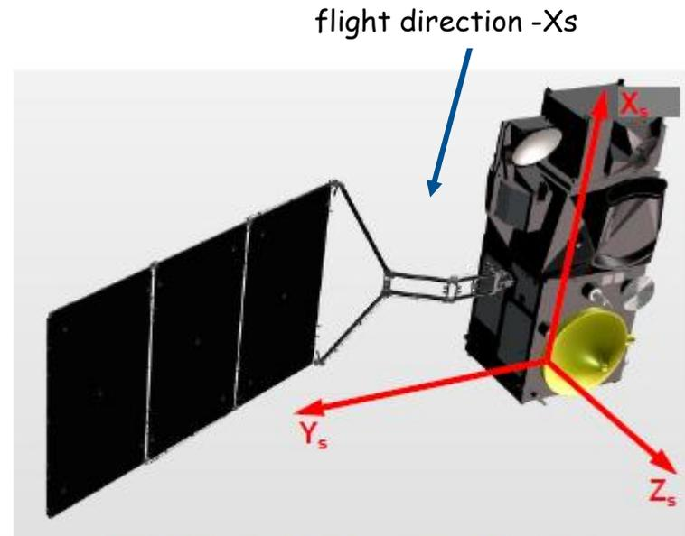
Figure 3-3 : Sentinel-3 in flight configuration and satellite reference axes
