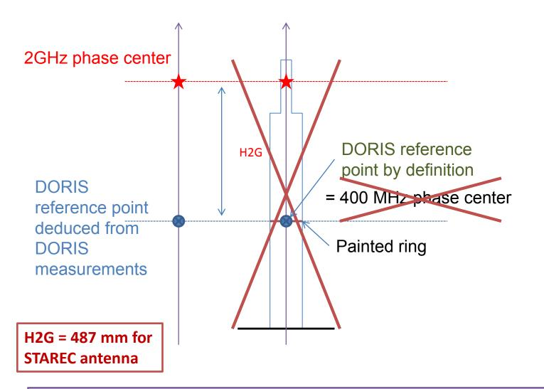
Recent radio frequency characterization performed by CNES concludes this geometry description of the STAREC antenna is wrong
