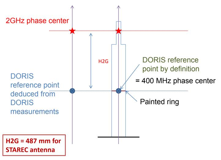
By definition. for a STAREC antenna. the DORIS reference point corresponds to the 400 MHz phase center. It is at the center of the red ring painted on the antenna.
