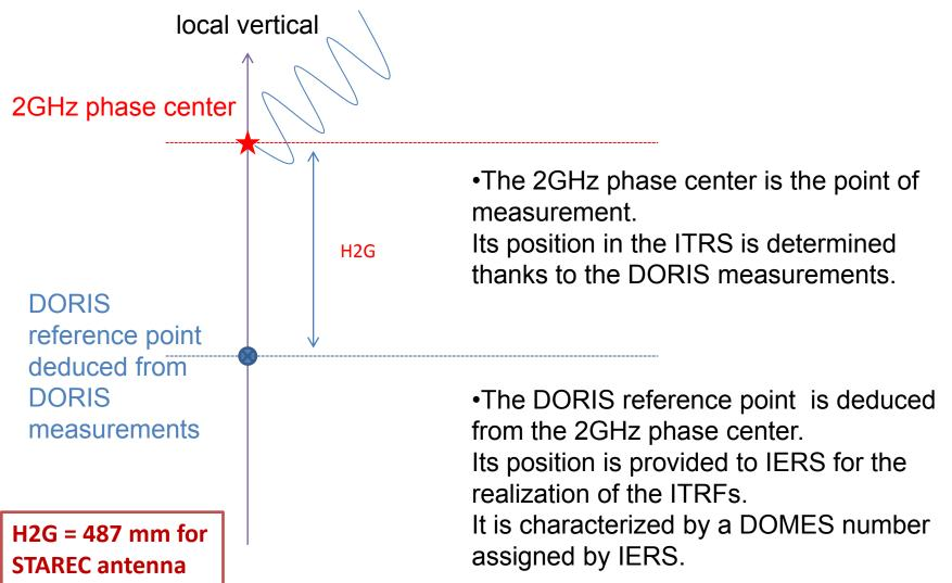
By construction. for a STAREC antenna. the DORIS reference point is located 487 mm under the 2GHz phase center. on the local vertical axis.
