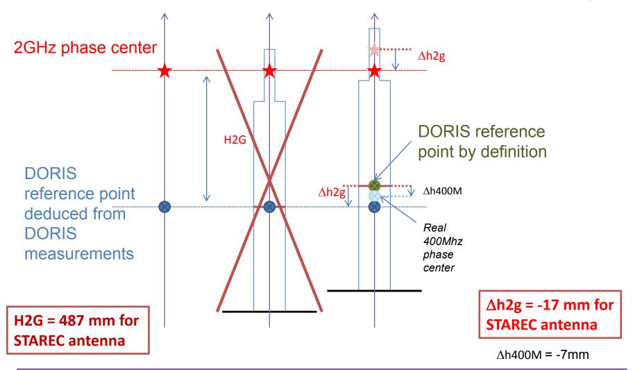
The 2GHz phase center is 17 mm under the supposed position and the 400Mhz phase center is 7 mm under the painted ring.
