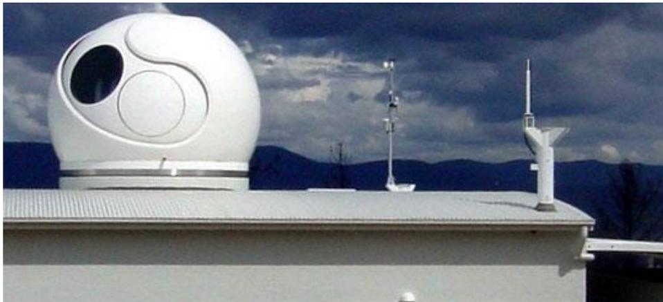
*Mount Stromlo Satellite Laser Ranging facility (left) and DORIS antenna (right)*
