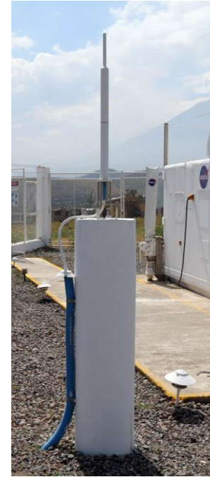
Type II. (ARFB, Arequipa) Concrete reinforced pillar extending up to 1.5 m depth.
