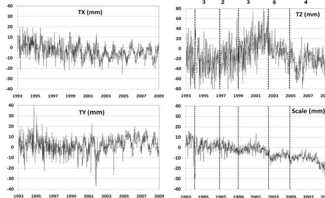
IDS-3 translation and scale parameters with respect to ITRF2005, dashes correspond to satellite constellation changes, upper right figures to the number of satellites
