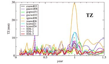
Mismodelling of solar radiation pressure induced systematic errors in the DORIS geocenter at the draconic period for TOPEX (118 days) and the SPOT and Envisat satellites (1 year). Fixing CR per satellite complete mission reduce this effect of leawd24 wrt leawd21 plots (Gobinddass, et al 2009)
