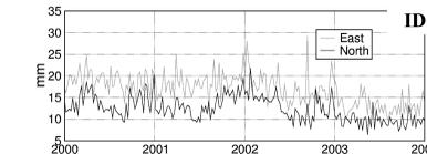
High residuals during 2001-2002 in IDS-1 are compensated by estimating drag coefficients every two hours and once an hour
