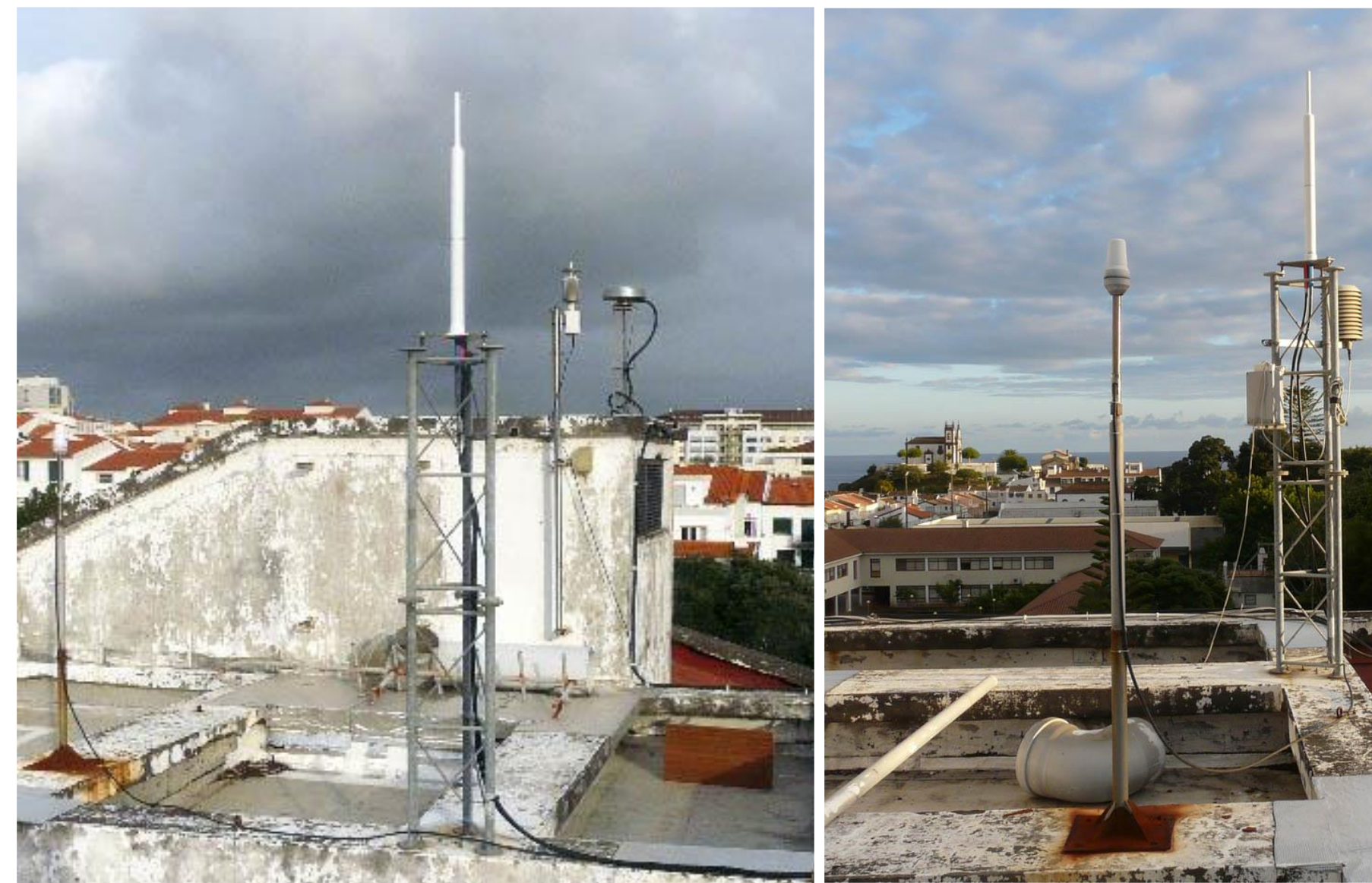
Figure 3 – The DORIS antenna "PDOC" with the GNSS "PDEL" in the background, part of the IGS network
