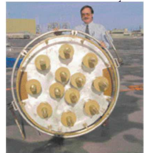
GPS Block IIA Antenna (Mader and Czopek, 2002)
