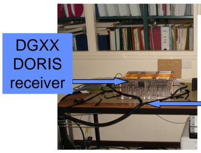
RF signals are injected through this wire via the antenna connection, and the Navigation is activated;
