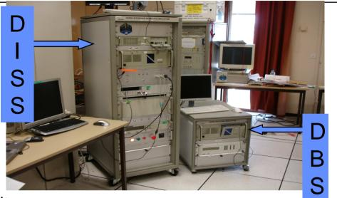
The DORIS Beacon Simulator (DBS) uses these numerical data (and also the Broadcasts uploads and/or attitude quaternions) to generate a RF analogic signal.
