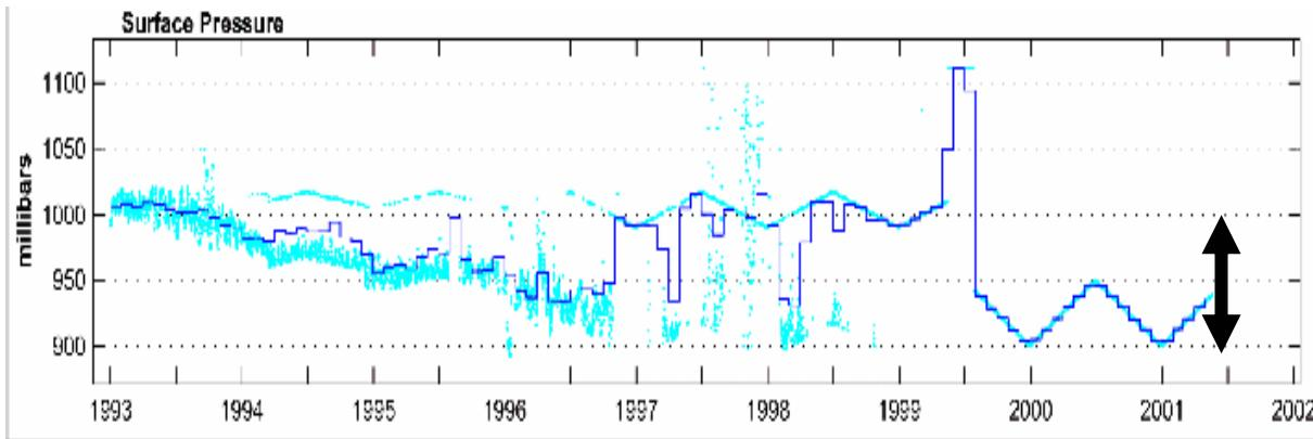
*100 mb drift of the pressure sensor
