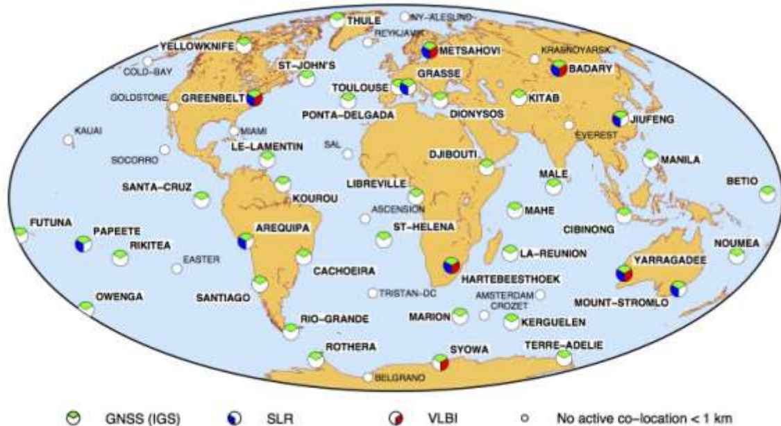
Fig. 1: The permanent DORIS network – 55 stations – and co-location with other IERS techniques (as on Dec. 2014).
