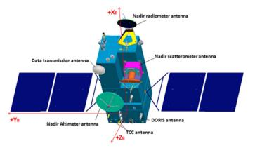
The attitude is a yaw steering attitude (like Jason or GPS satellites) yaw rotation around the radial axis (z)
