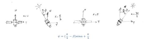
Oscillation at orbital period around the normal axis  ${\cal N}$
