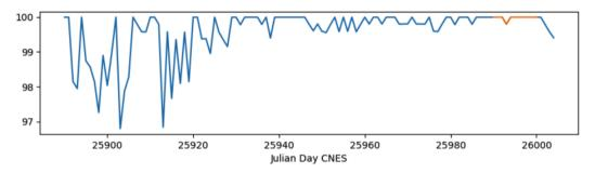
FIGURE : Fixing rates of GPS ambiguities for HY-2C.
