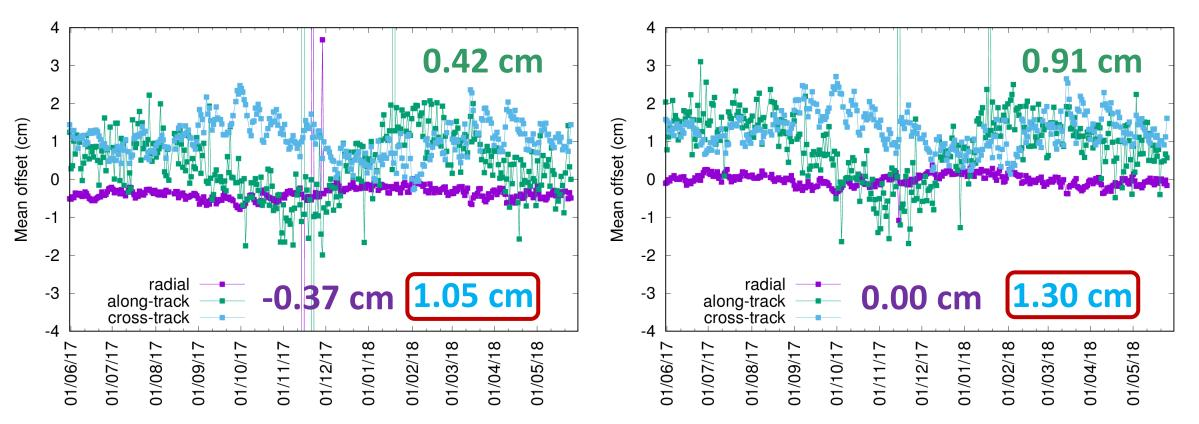
Daily mean offsets (m) between S-3A DORIS orbits and CLS/GRGS orbits (left) and QWG combined orbits (right)
