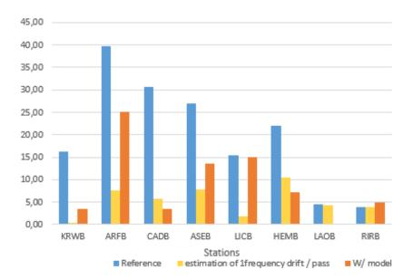
Mean of the vertical positioning over ~40 cycles (cm)
