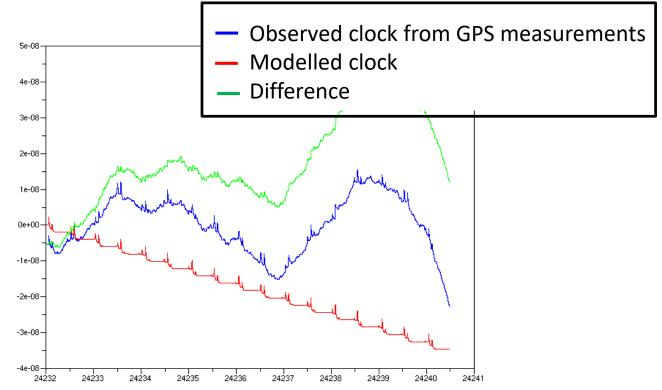
Note : the drift coming from the integration of the model is small enough not to perturb the time tagging. (3 10<sup>-8</sup> sec / 9 days, i.e 7mm over 1 pass)
