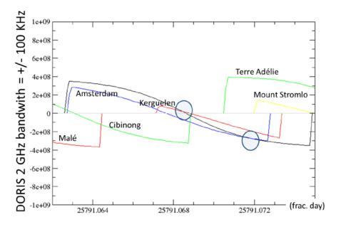
DOPPLER CROSSINGS OVER YARAGADEE (IN BLACK), NO SHIFT (K=0) The figure opposite is done with Yaragadee frequency shifted. On this descending pass we have suppressed every crossing by using a K=50 frequency shift. Of course, it is necessary to check also other passes, including ascending passes.
