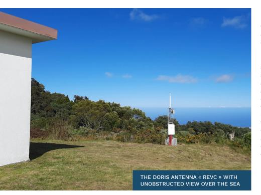
Another strength of this site is the **colocation with the GNSS station "REUN",** installed and managed by IGN since 1998 and part of the IGS network. The recent site survey performed by IGN during the DORIS station renovation provided new tie vectors in order to contribute to the next realization of the International Terrestrial Reference Frame (ITRF2020).
