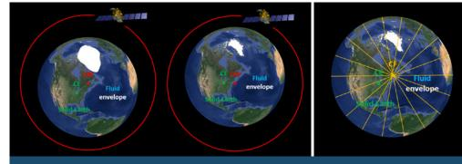
MOTION OF THE CENTER-OF-MASS (CM) OF THE WHOLE EARTH (SOLID BODY AND FLUID ENVELOPE) WITH RESPECT TO THE CENTER-OF-MASS (CE) OF ITS SOLID PART [LEFT, CENTER] AND CENTER-OF-FIGURE (CF) [RIGHT].
