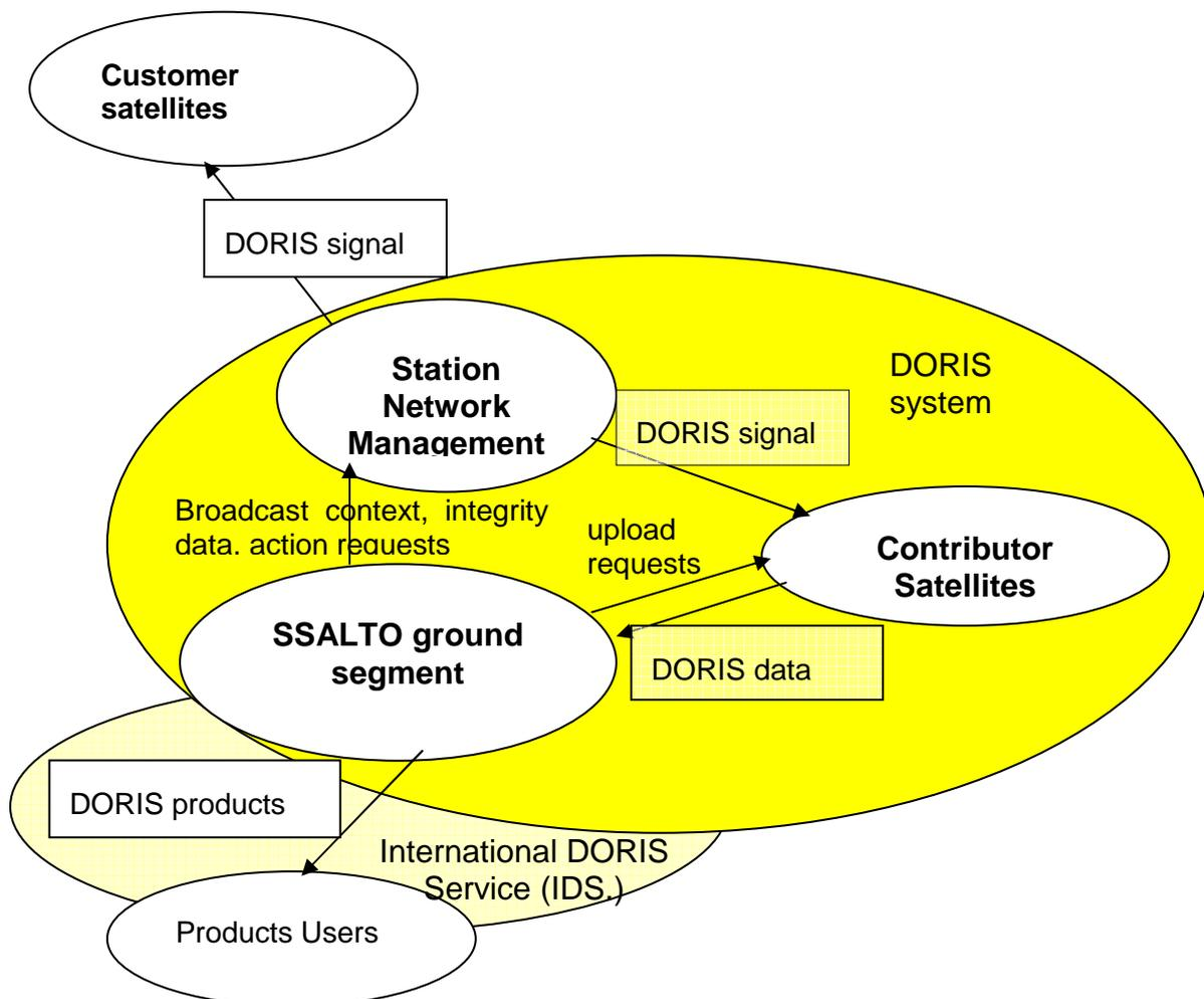
Fig.4 – The DORIS system : external and internal connections
