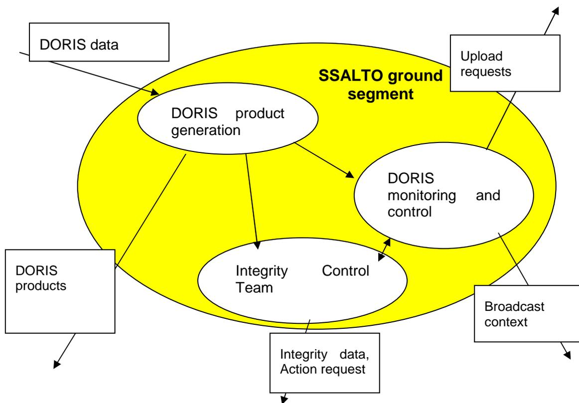
**Fig. 11 – DORIS monitoring and ground processing**
