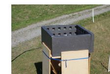
Attenuation effect of absorber plates at site C1 on RTW. 3 plates (setup left) reduce the signal by 12-20 dB.
