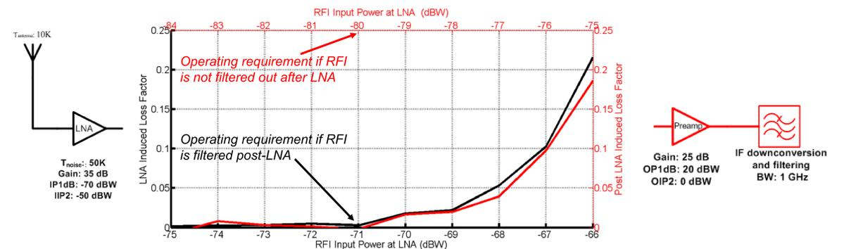
Figure 4. Dependence of correlation losses on the input RFI level when the LNA is overdriven and when the post-LNA hardware is overdriven
