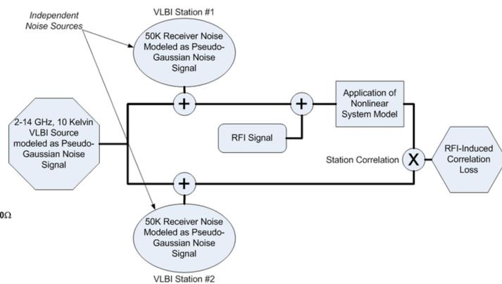
Figure 2. Block diagram outlining VLBI signal simulation used to assess station correlation loss
