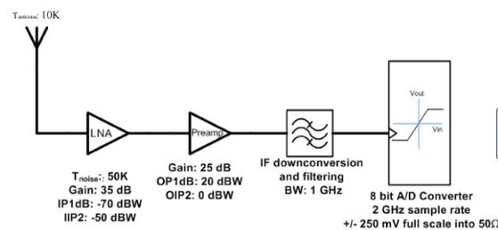
Figure 1. VLBI receiver chain model
