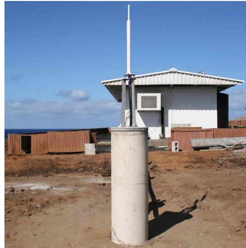
Type II (24%): custom-made tripod on concrete pillar
