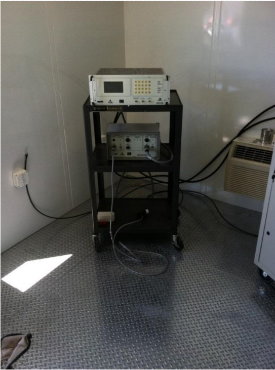
Figure 1: DORIS Beacon setup in GNSS Equipment Building, A temperature controlled room
